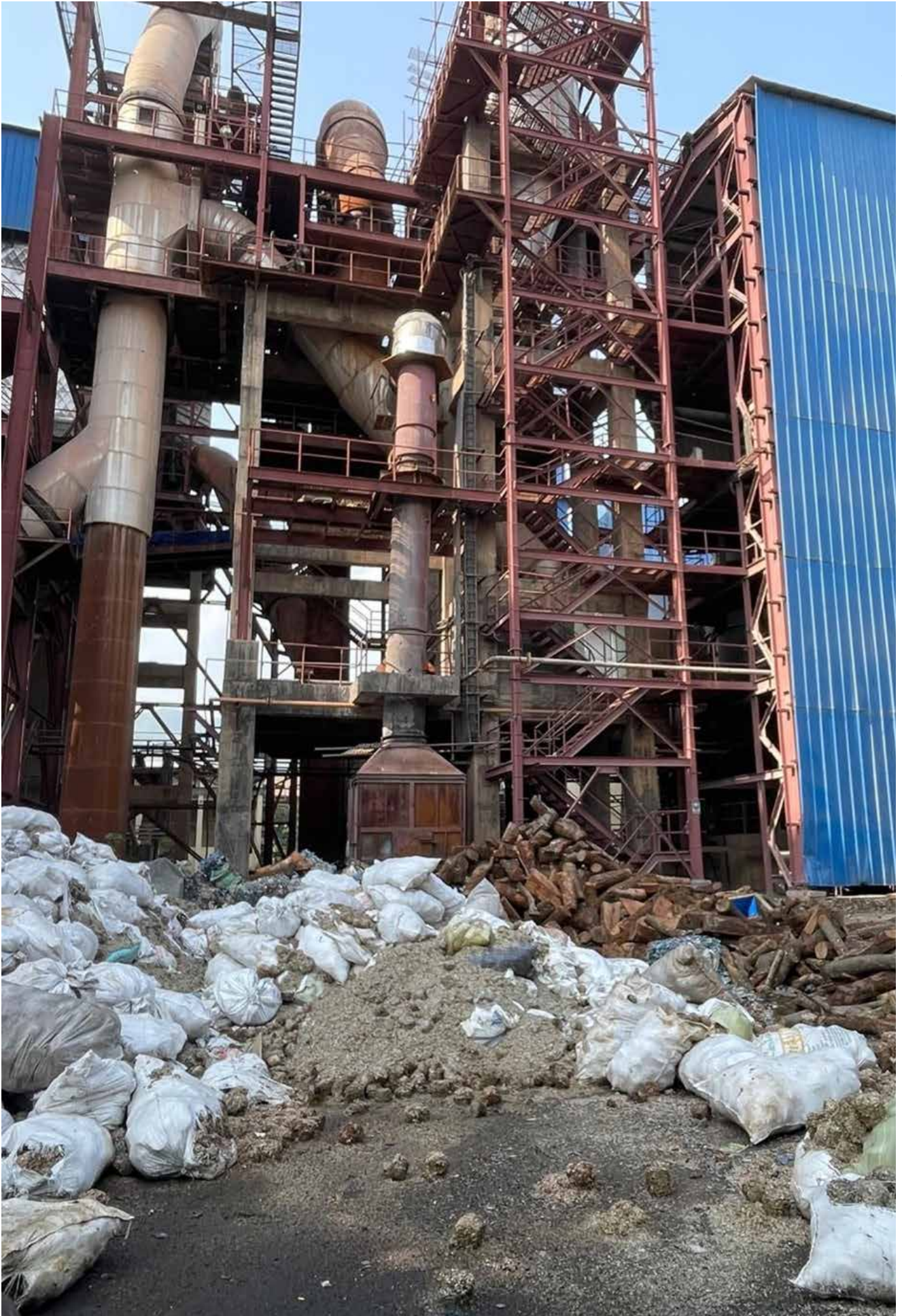
A cement factory using low-value plastics as refuse-derived fuel in a controlled way.
