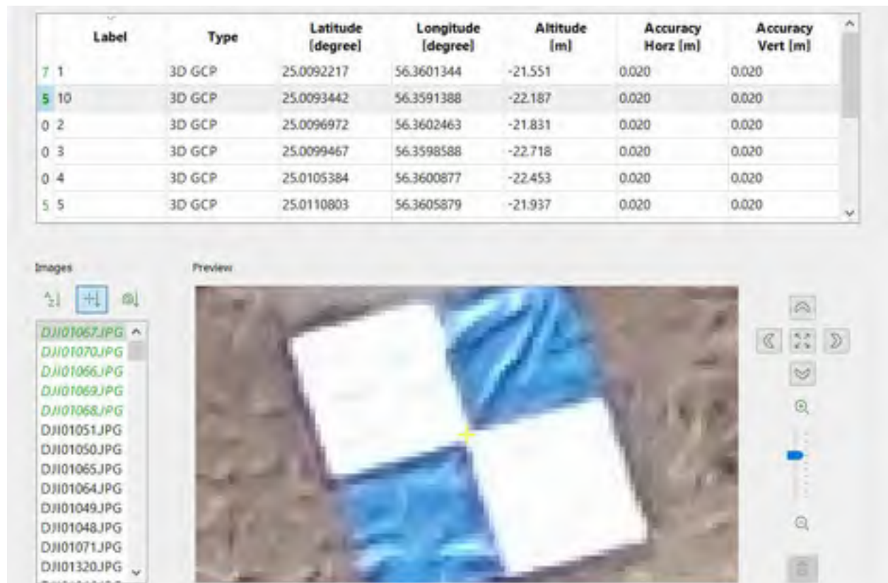
Figure 16. The Basic Editor tool used to tag each GPS point back to the GCPs on images taken by the drone. At least 3 GCPs need to be tagged to georeference an image. The GCPs should be placed in the corners and centre of the study area for the best georeferencing results.
