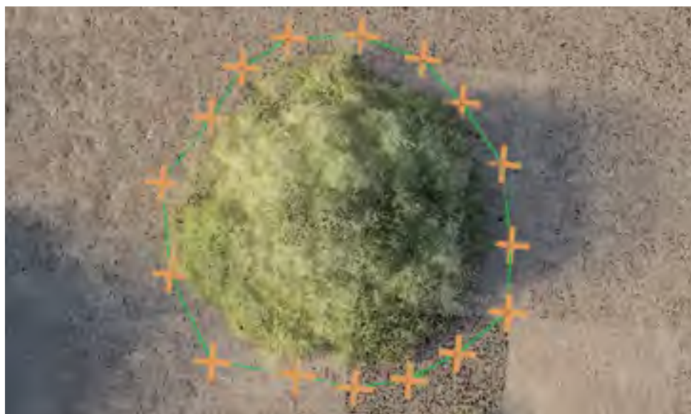
Figure 21. New Volume shape around a tree feature in the Pix4D rayCloud editor to initiate volume calculations.
