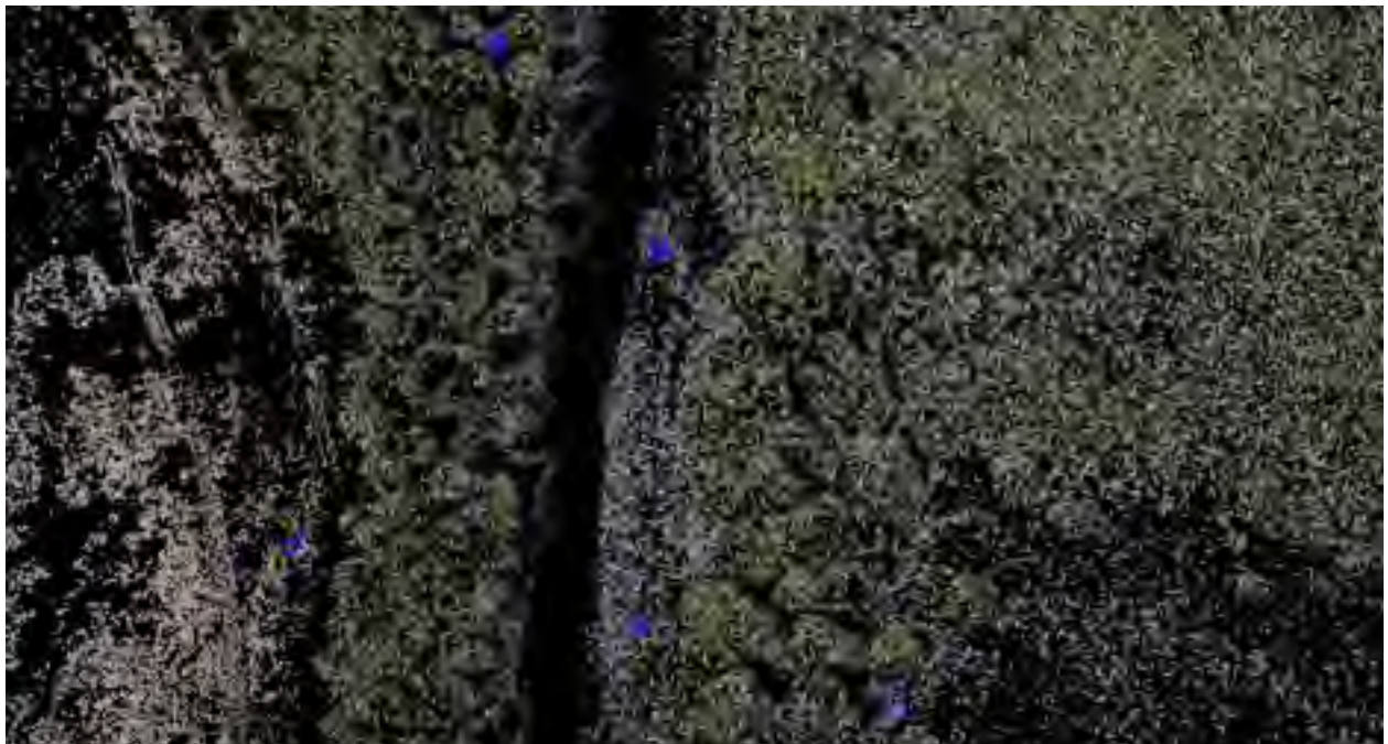
Figure 17. 3D image of the study area with ground control points represented in blue. These points were used to georeferenced the 3D model in space to its accurate x, y, and z position.
