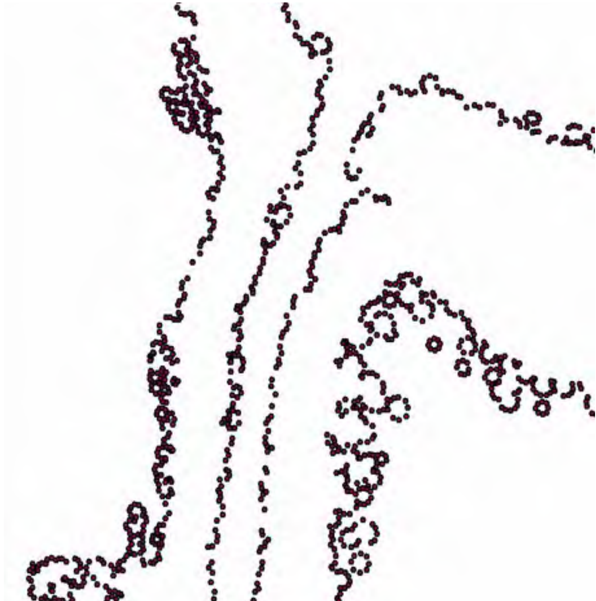
Figure 28. Points created around the mangrove tree features from the tree polygon shapefile. Using the Zonal Statistics tool, we assign elevation values from the DSM to each point.
