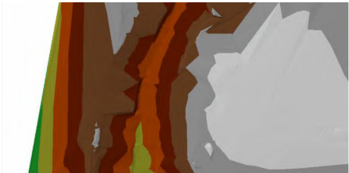
Figure 29. TIN output created using the Create Tin tool in ArcGIS that extrapolates the elevation values from the points created in figure 18 across space.
