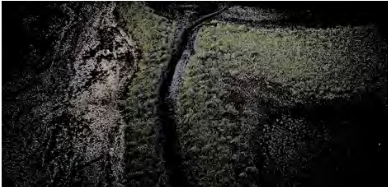
Figure 13. Rough 3D model created through the Initial Processing step. Brighter areas in the center of the image have a higher point density and show location with a higher image overlap.
