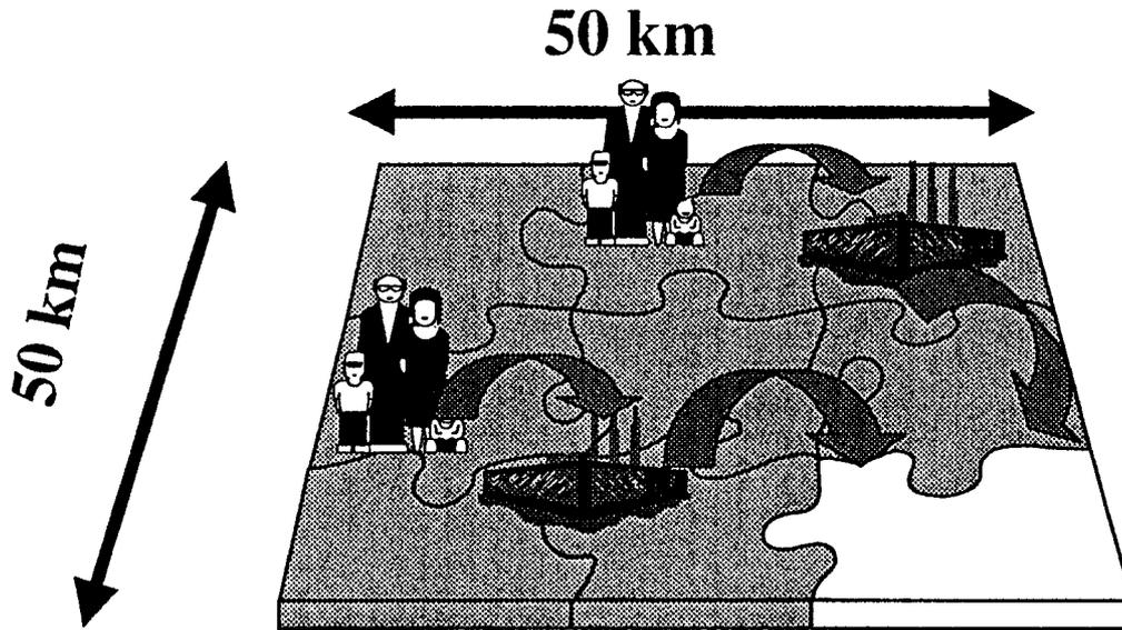
Figure 4. Flow of nitrogen load within a grid cell from the human population via sewage treatment to natural wetlands. The white area represents the natural wetland area within a grid cell.
